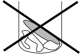
Do not stack the laundry one side
